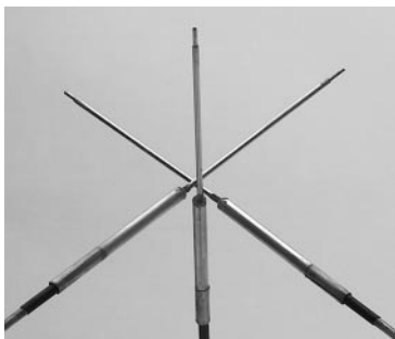
Figure 3 Tri-polarized antenna (tripole). The composite structure is composed of three orthogonal sleeves 12 with their feed points collocated at the centre of the image. Each has two variable length segments which are adjusted to efficiently couple radiation to its transmission line. The three antennae together can create an arbitrary vector electric dipole moment at the transmitter, as well as function as detectors of the vector electric field at the receiver.
