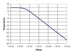
For noisy oscillators, the phase noise will again always be less than 0 dBc/Hz, but this gives us a spectral line width that is greater than 1 Hz. The phase noise goes flat below  $f_{HW}$ , showing the
