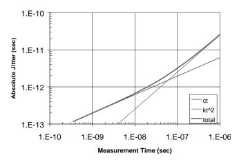
Ignoring 1/f noise gives reasonable results when the jitter measurement time is less the reciprocal of the 1/f noise corner frequency.
