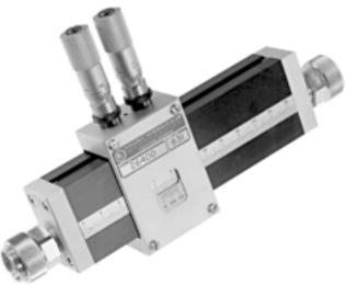
The double probe tuner utilizes two variable reactance elements to achieve an extremely high matching capability over a broad frequency range. In normal operation, only one probe is required to match an impedance having a VSWR of 6:1 or less. Both probes are required only at the lowest frequencies, as much higher VSWR's can generally be matched over most of the operating band.
